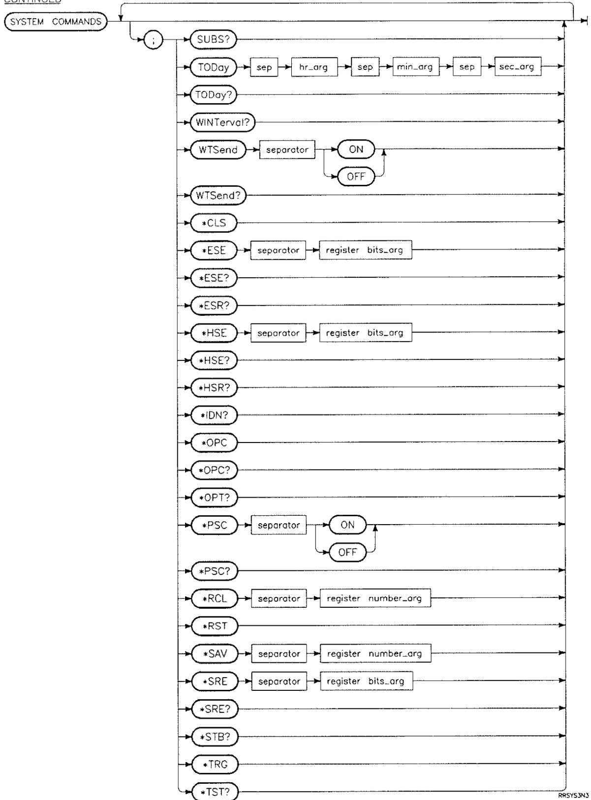
Figure 5-1. System Command Syntax Diagram (3 of 3)
