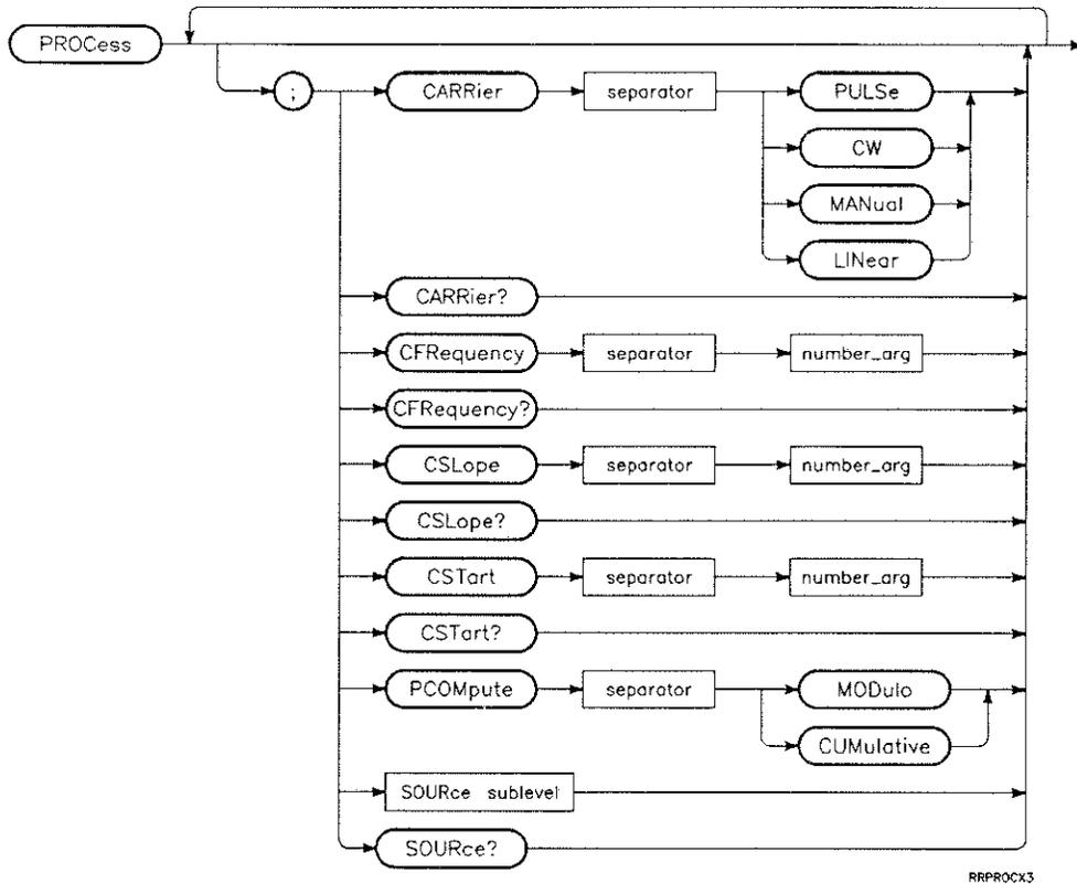
*Figure 5-13. PROCEss (MATH) Subsystem Syntax Diagram*
