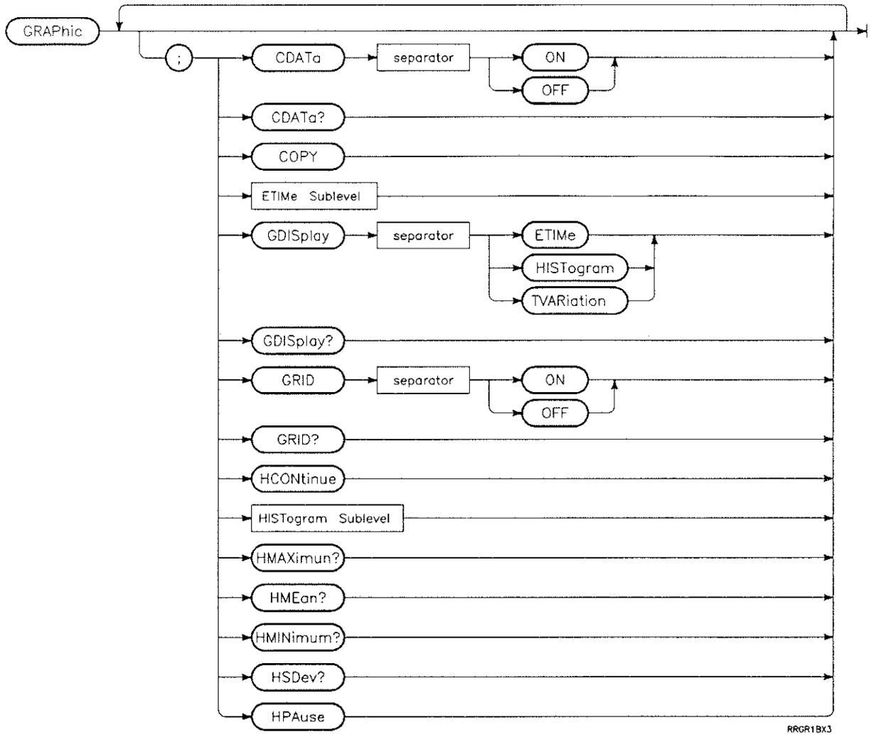
Figure 5-4. GRAPHic Subsystem Syntax Diagram (1 of 4)
