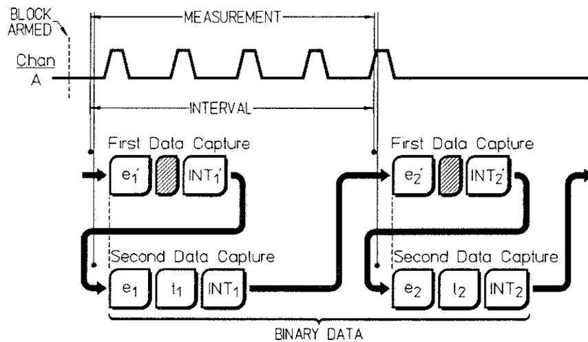
Figure 11-A. Totalize Measurement on Channel A with Interval Sampling Arming Mode Showing Corresponding Binary Output
