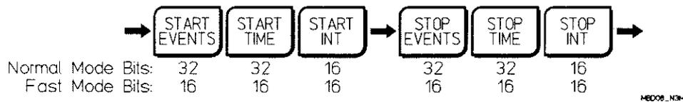
*Figure 5B-B. Format 5B Binary Output*
