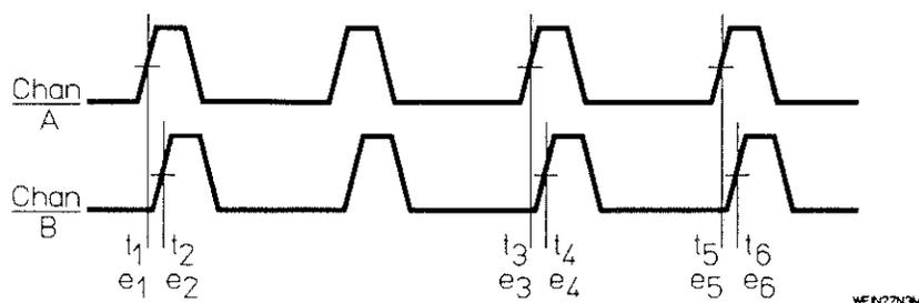
Figure 10B-I. Phase Example Signal Showing Time and Event Stamp Measurement Points
