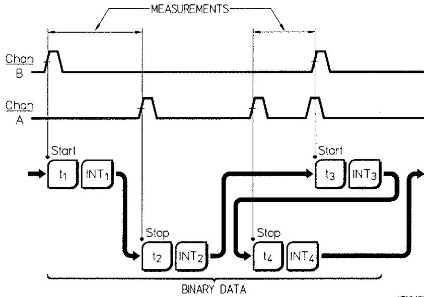
Figure 4B-A. Time Interval Measurement on Channel A  $\rightarrow$  B with Automatic Arming Mode Showing Corresponding Binary Data Output
