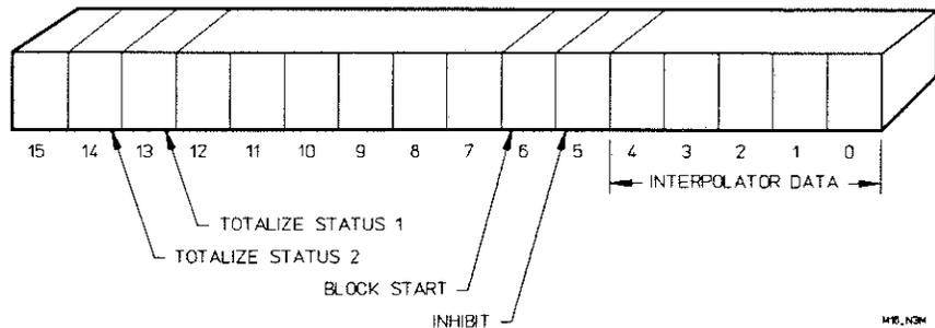
Figure 3-5. 16-bit Interpolator/Status Field
