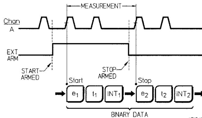
Figure 5A-A. Frequency Measurement on Channel A with Externally Gated Arming Mode Showing Corresponding Binary Data Output
