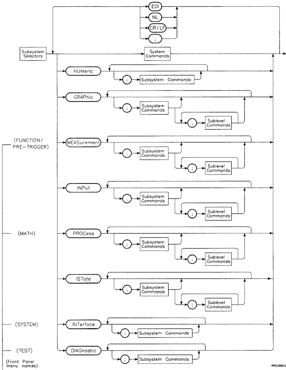
Figure 4-4. Top Level Command Syntax Diagram
