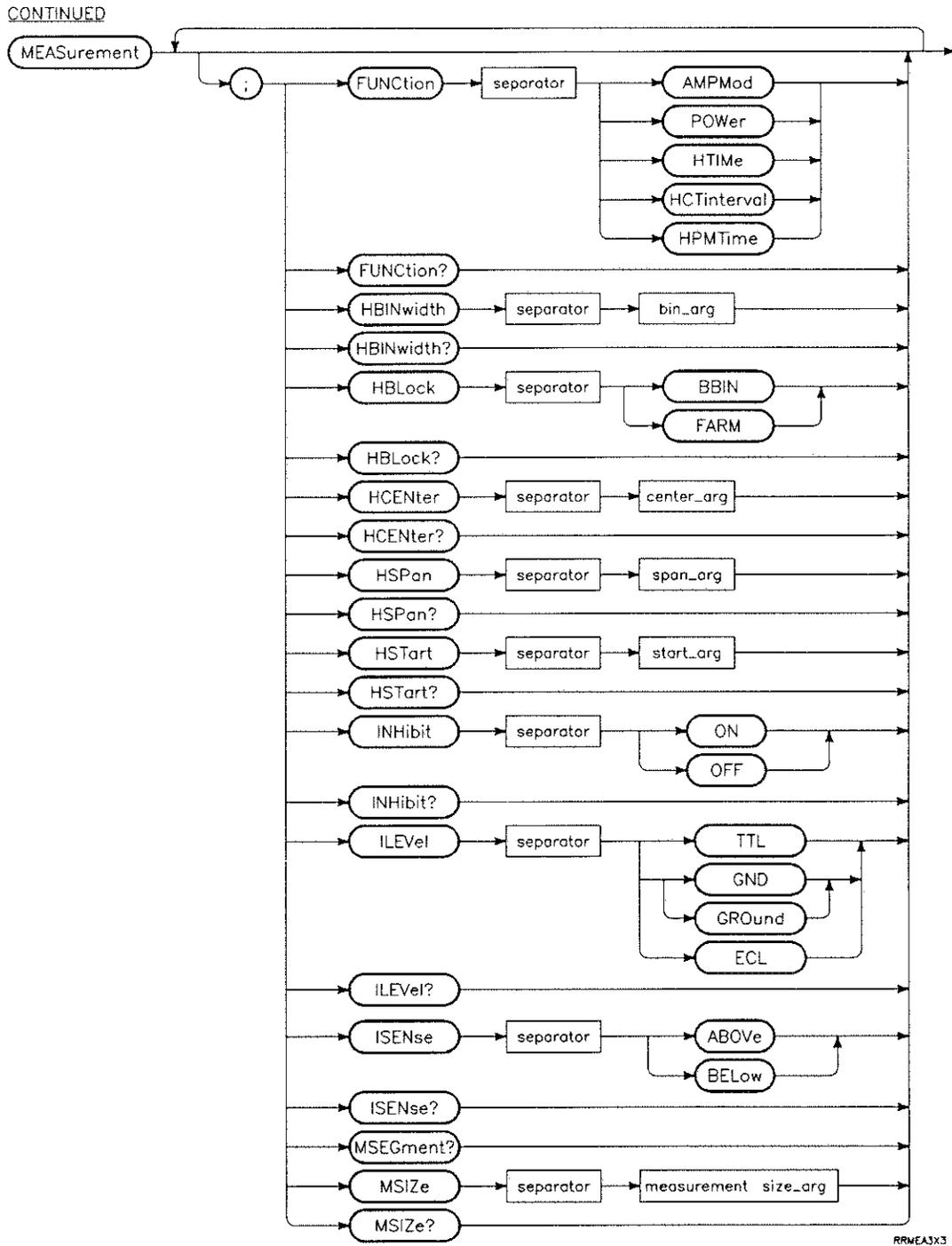
Figure 5-8. MEASurement Subsystem (FUNCTION/PRE-TRIGGER) Syntax Diagram (3 of 4)
