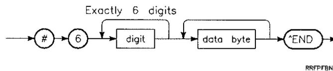
Figure 2-4. Floating Point Format Block Message Syntax
