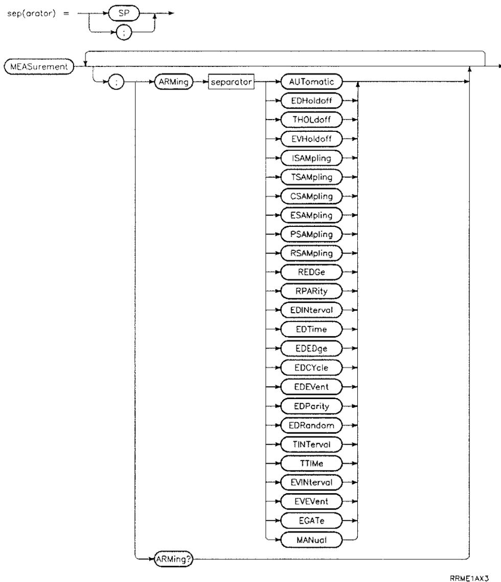
Figure 5-8. MEASurement Subsystem (FUNCTION/PRE-TRIGGER) Syntax Diagram (1 of 4)
