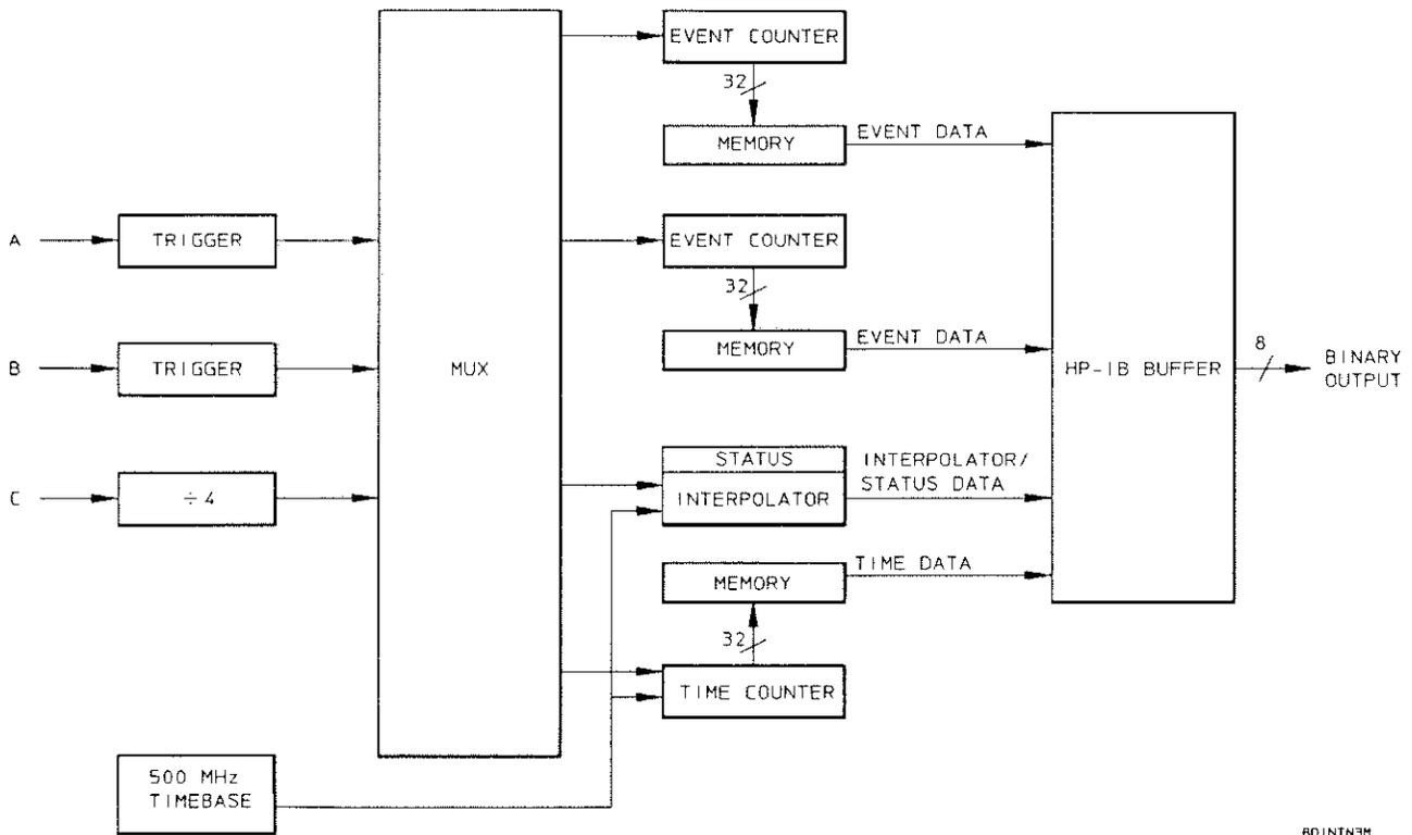
Figure 3-1. Simplified Block Diagram of HP 5373A Measurement Section with Binary Output
