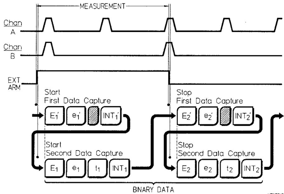
Figure 15-A. Totalize Measurement on Channels A and B with Externally Gated Arming Mode, Showing Corresponding Binary Output
