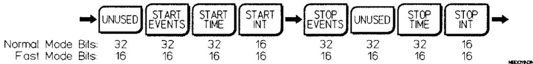
Figure 10C-B. Format 10C Binary Output
