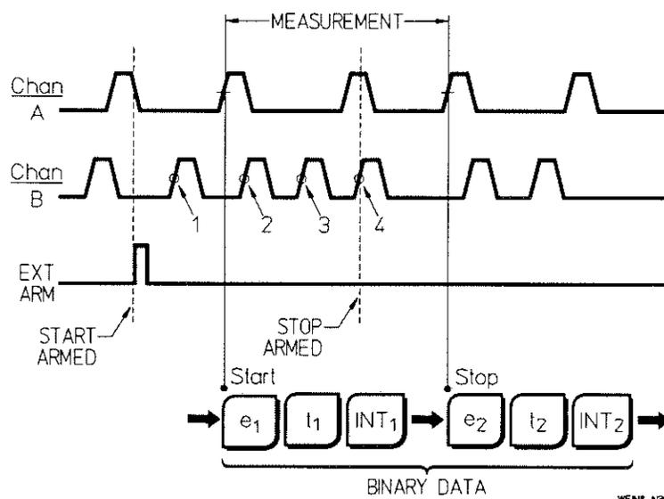
Figure 5B-A.  $\pm$ Time Interval Measurement on Channel A with Edge/Event Arming Mode Showing Corresponding Binary Data Output
