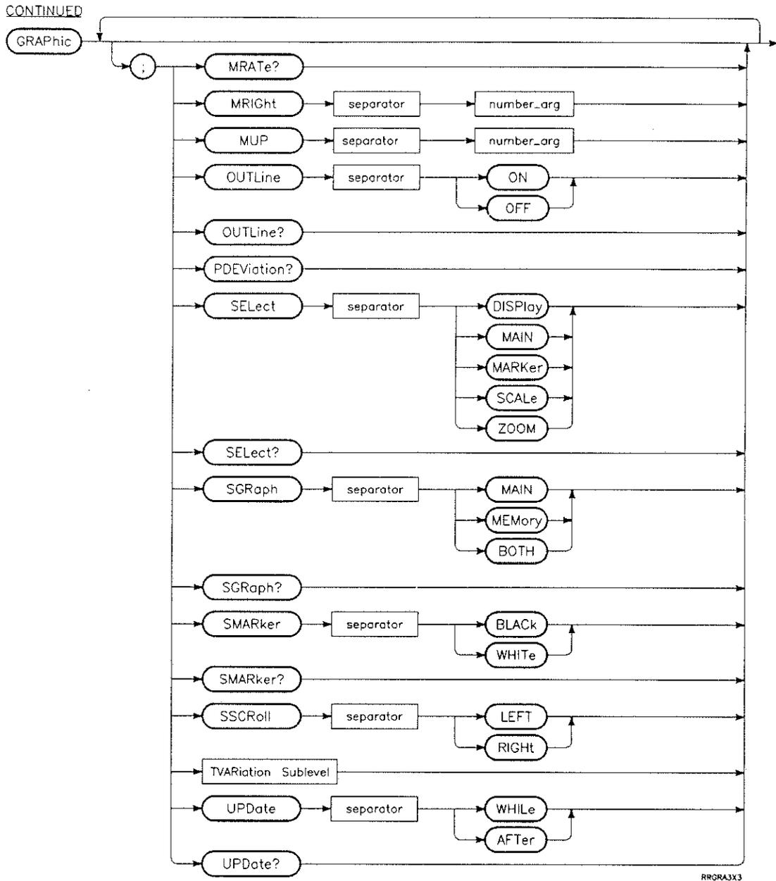
Figure 5-4. GRAPHic Subsystem Syntax Diagram (3 of 4)
