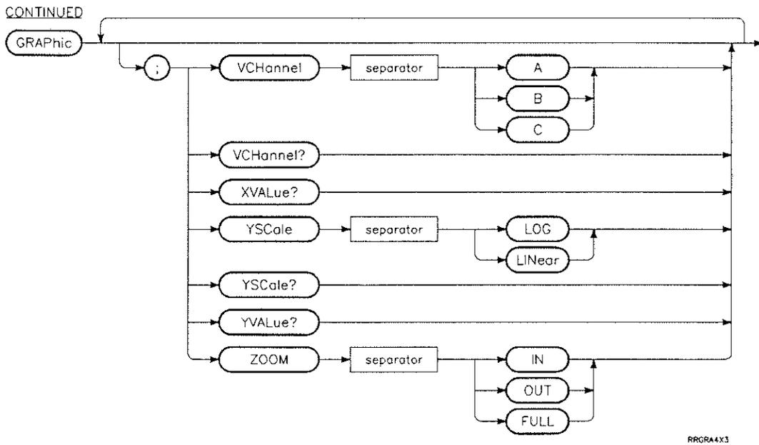
Figure 5-4. GRAPHic Subsystem Syntax Diagram (4 of 4)
