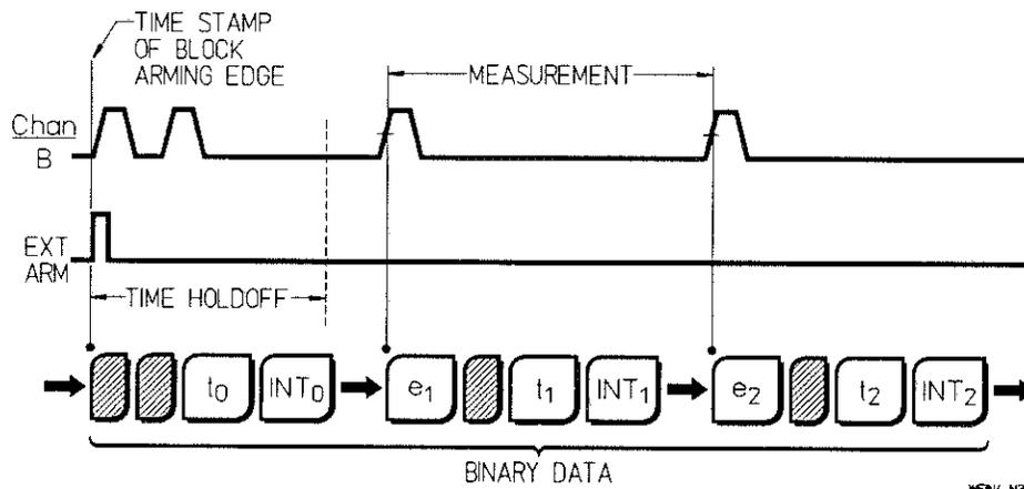
Figure 3-A. Frequency Measurement on Channel B with Time Holdoff Arming Mode Showing Corresponding Binary Data Output
