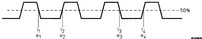
Figure 10B-H. Negative Pulse Width Example Signal Showing Time and Event Stamp Measurement Points
