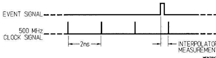
Figure 3-2. Interpolation Between 2 ns Clock Pulses
