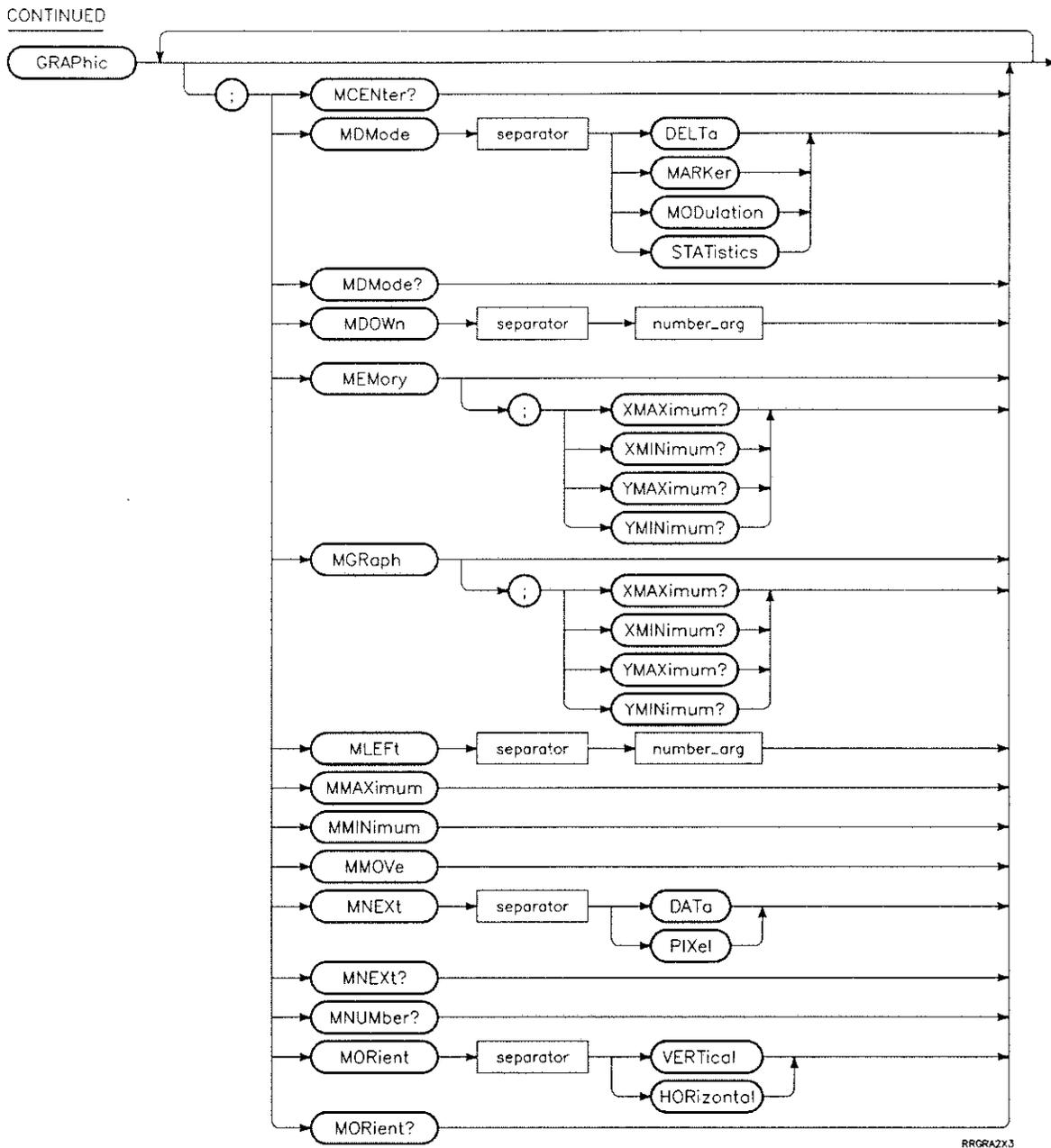
Figure 5-4. GRAPHic Subsystem Syntax Diagram (2 of 4)
