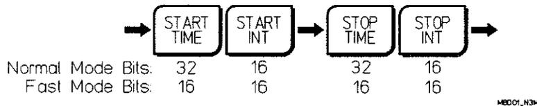
Figure 4B-B. Format 4B Binary Output
