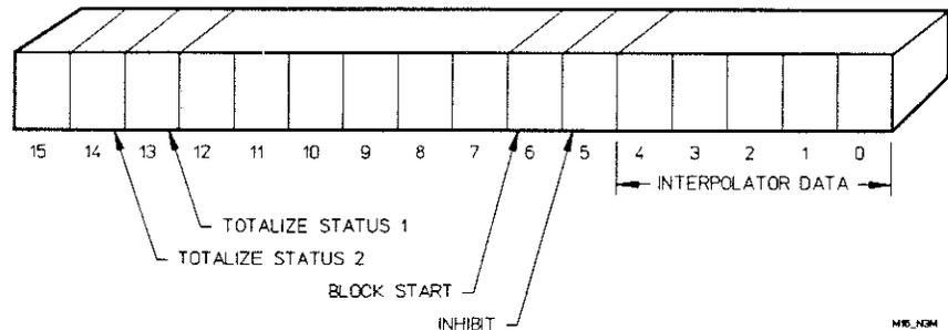
Figure 3-6. 16-bit Interpolator/Status Field
