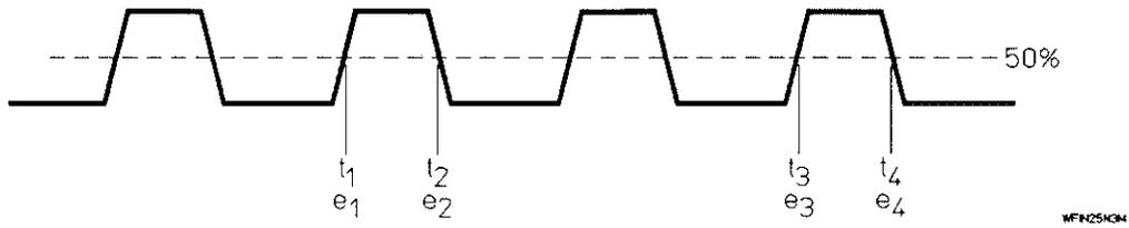
Figure 10B-G. Positive Pulse Width Example Signal Showing Time and Event Stamp Measurement Points
