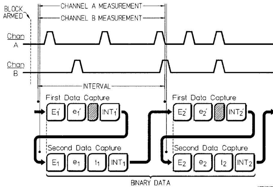
Figure 13-A. Totalize Measurement on Channel A and B with Interval Sampling Arming Mode Showing Corresponding Binary Output
