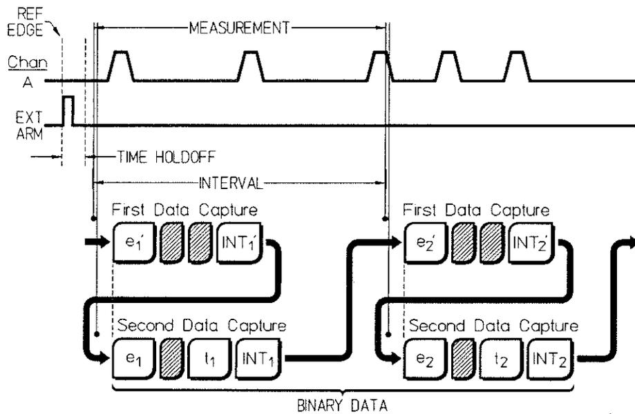
Fig 12-A. Totalize Measurement on Channel A with Time/Interval Arming Mode Showing Corresponding Binary Output.
