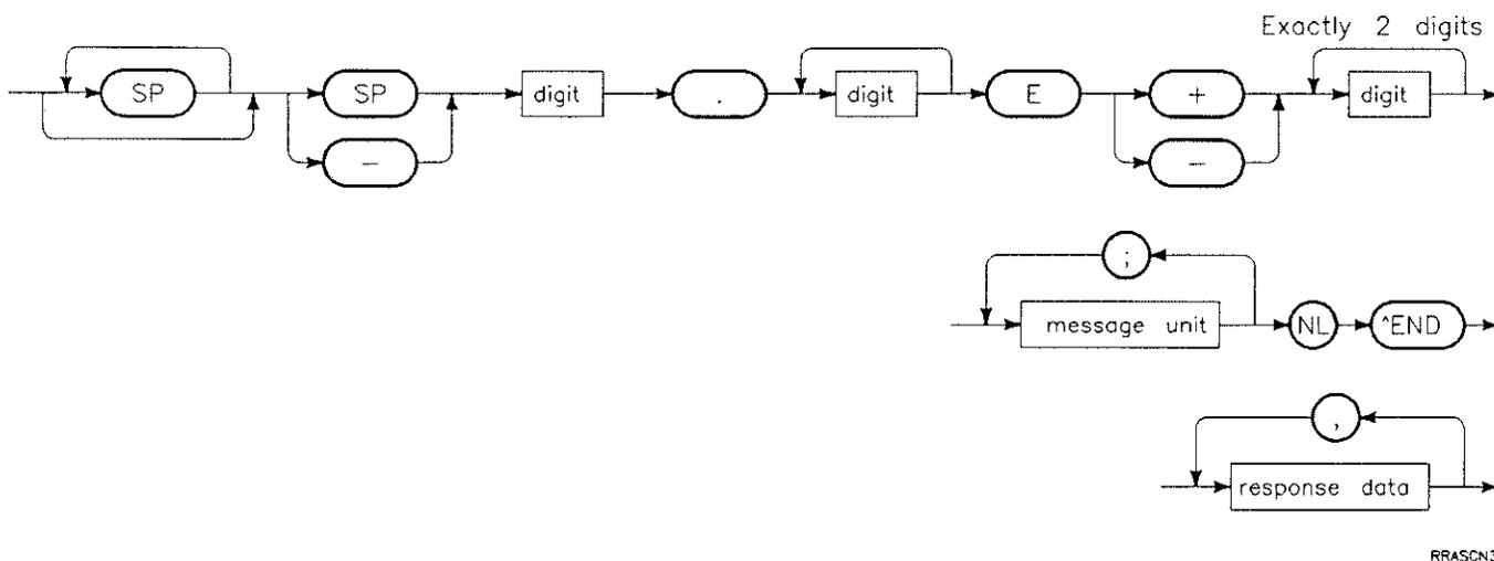
Figure 2-3. ASCII Measurement Result Syntax Diagrams
