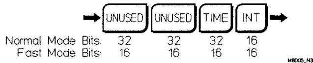
Figure 3-B. Format 3, First Sample in Each Block
