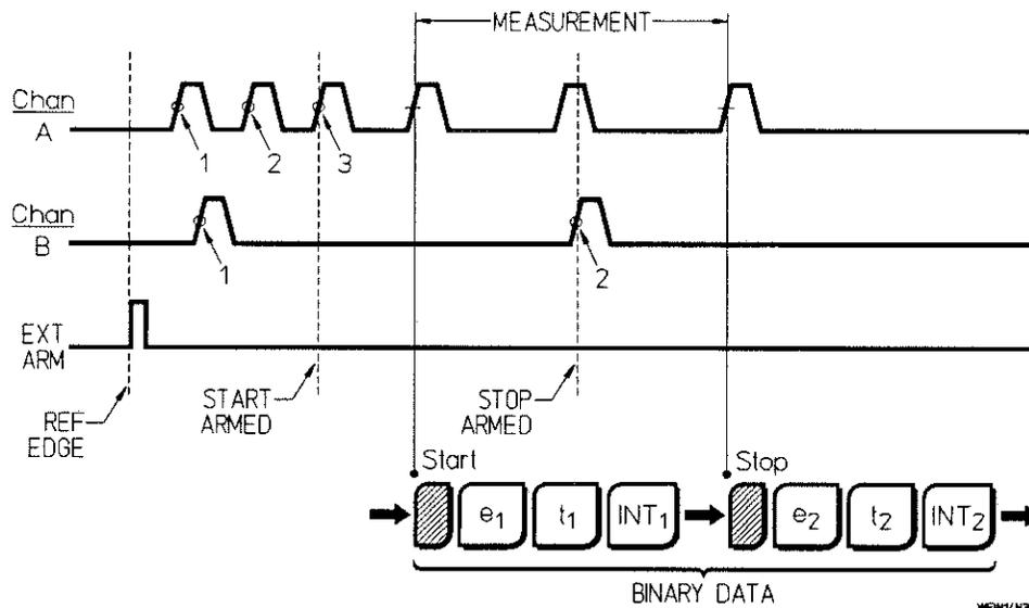
*Figure 10D-A. Frequency Measurement on Channel A with Event/Event Arming Mode Showing Corresponding Binary Output.*
