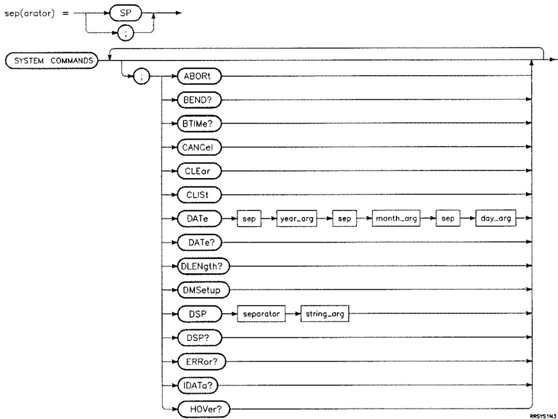
Figure 5-1. System Command Syntax Diagram (1 of 3)
